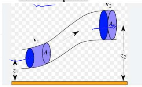
$$\frac{P}{\gamma} + \frac{U_1^2}{29} + Z_1 = \frac{P_2}{\gamma} + \frac{V_2^2}{29} + Z_2 \rightarrow \%$$
