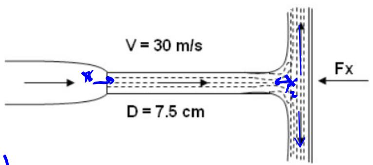
$$\therefore f_x = -f_r = \rho Q (v_2 - v_1)$$
