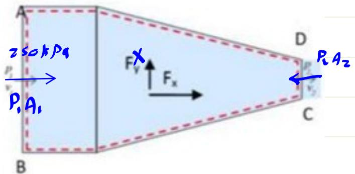
$$P = 250 + 10^3 \text{ Pa} , Q = 1 + 10^{-3} \text{ m}^3/\text{s} , d_1 = 0.025 \text{ m}$$
