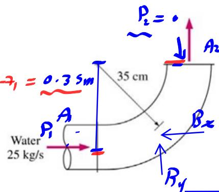
$$\begin{aligned} A_1 &= A_2 \\ V_1 &= V_2 \\ Q &= A_1 V_1 = A_2 V_2 \end{aligned}$$
