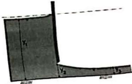
1. A partially open sluice gate in a 5-m-wide rectangular channel carries water at 10 m<sup>3</sup>/s. The upstream depth  $y_1$  is 2.5 m. Find the downstream depth,  $y_3$  and Froude number.
