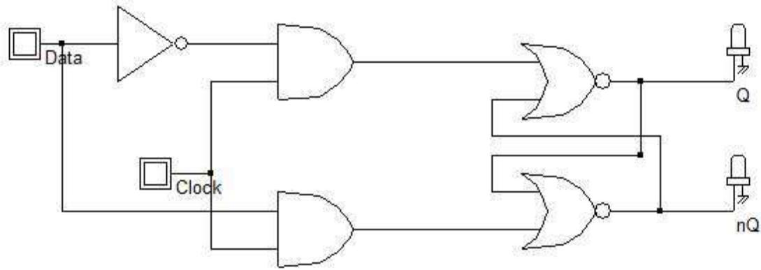
When performing the logic simulation  $Q$  and  $nQ$  starts with an undetermined state. Once the clock is active  $Q$  and  $nQ$  turn to a deterministic state, as the data input  $D$  is transferred to  $Q$ , and its opposite to  $nQ$ . When clock returns to level  $0$ , the latch keeps its last value.
