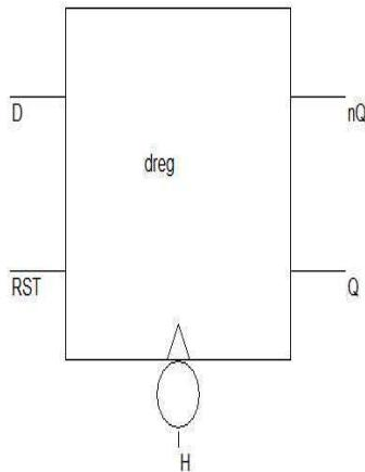
Notice that the triangle at the clock input recalls the sensitivity of outputs Q and nQ to the edge of the clock. The circle indicates that this Dreg cell is sensitive to a fall edge of the clock.
